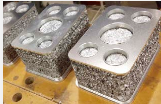
Skin structure with composite aluminium foam installed
